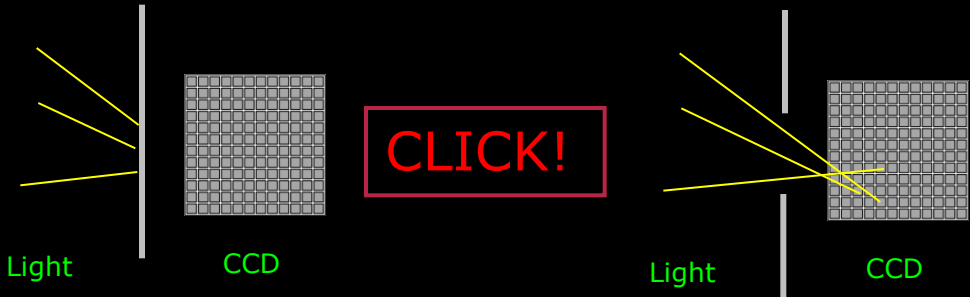
The shutter opens and the CCD is hit by light
